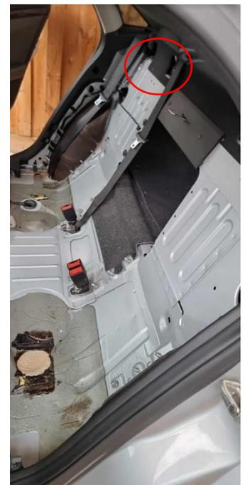
4. AVOID bunching your power wire as they can get hot. I wrapped mine around the empty chassis directly behind the seat (see photo of back seat: [red circle](#))
